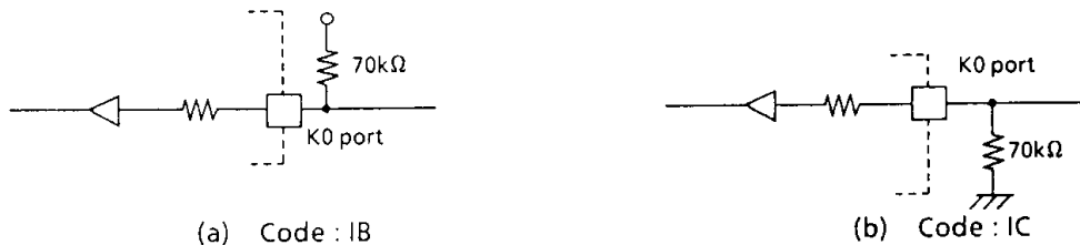
Figure 2. I/O code and external circuitry
