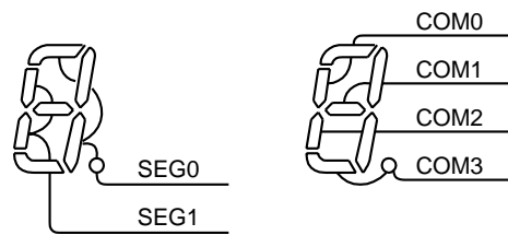
Figure 15-6 Example of COM, SEG Pin Connection (1/4 Duty)
