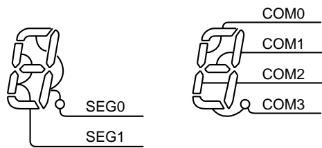
Figure 15-6 Example of COM, SEG Pin Connection (1/4 Duty)
