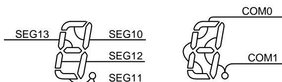
Figure 15-6 Example of COM, SEG Pin Connection
