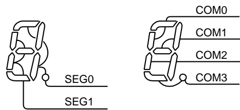
Figure 13-6 Example of COM, SEG Pin Connection (1/4 Duty)
