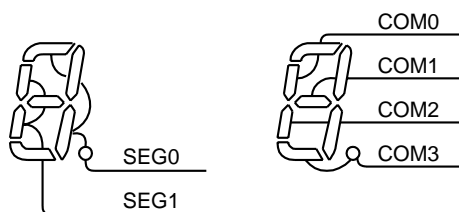
Figure 13-6 Example of COM, SEG Pin Connection (1/4 Duty)
