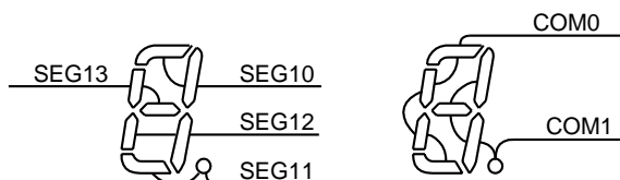
Figure 15-6 Example of COM, SEG Pin Connection
