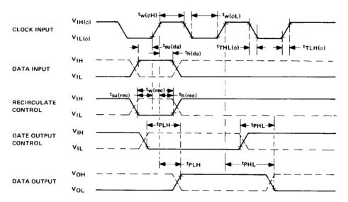
NOTE: Measurements are made at 90% (high) and 10% (low) timing points.
