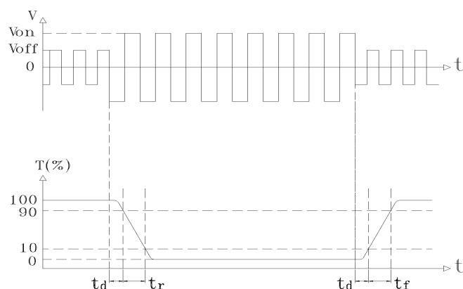
$$\text{Turn on time: } t_{on} = t_d + t_r \quad \text{Turn off time: } t_{off} = t_d + t_f$$
