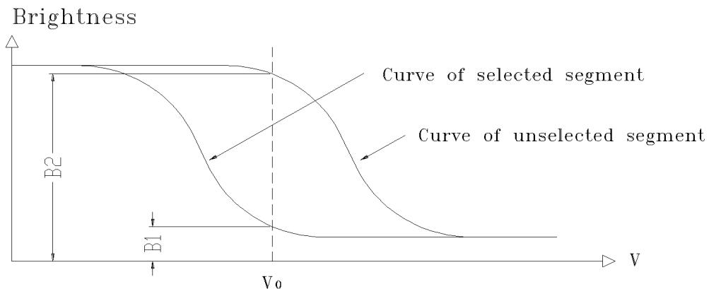
$$\text{Contrast Ratio} = B2/B1 = \frac{\text{unselected state brightness}}{\text{selected state brightness}}$$
