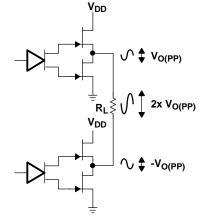
Figure 31. Differential Output Configuration
