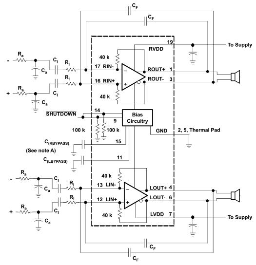
A. C<sub>(LBYPASS)</sub> and C<sub>(RBYPASS)</sub> are optional.
