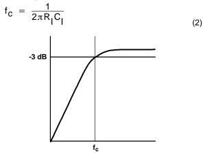
The value of C<sub>1</sub> is an important consideration. It directly affects the bass (low frequency) performance of the circuit. Consider the example where R<sub>1</sub> is 10 k $\Omega$  and the specification calls for a flat bass response down to 100 Hz. Equation 2 is reconfigured as Equation 3.
