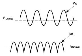
Figure 33. Voltage and Current Waveforms for BTL Amplifiers
