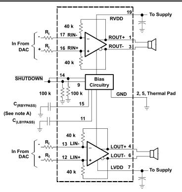
A. C<sub>(LBYPASS)</sub> and C<sub>(RBYPASS)</sub> are optional.
