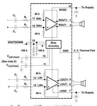
A.  $C_{(LBYPASS)}$  and  $C_{(RBYPASS)}$  are optional.
