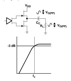
Figure 32. Single-Ended Output and Frequency Response
