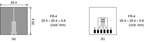
(b) Device mounted on a glass-epoxy board (b)
