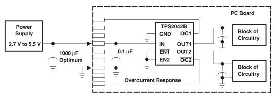
Figure 37. Typical Hot-Plug Implementation (Example, TPS2042B)
