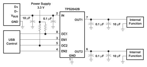
Figure 32. High-Power Bus-Powered Function (Example, TPS2042B)
