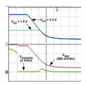
Figure 42. Simultaneously Tracking Down
