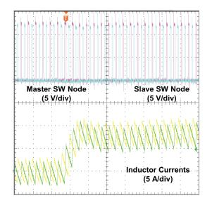
Figure 45. Current Balance at 0 A to 16 A Load Step Up, 2.5 A/ $\!\mu s$  Slew Rate
