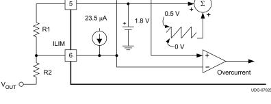
Figure 25. Current Sense Architecture
