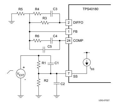
Figure 24. Tracking Setup
