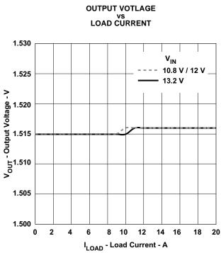
Figure 39. Output Load Regulation
