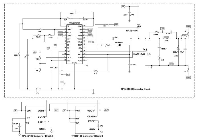
In Figure 43, Block I and Block II are configured as master and slave respectively.
