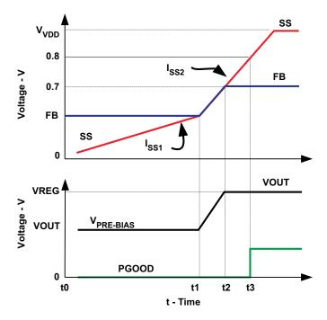
Figure 22. Soft-Start Waveform for Pre-Biased Outputs
