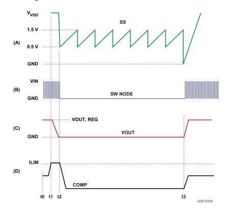
Figure 26. Hiccup Recovery From Faults
