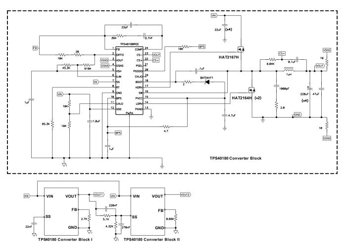
Figure 40. Additional Application Circuit I: Simultaneous Tracking with TPS40180 Devices
