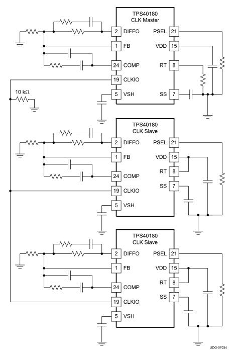
Figure 32. Phase Share Multiple Output Configuration
