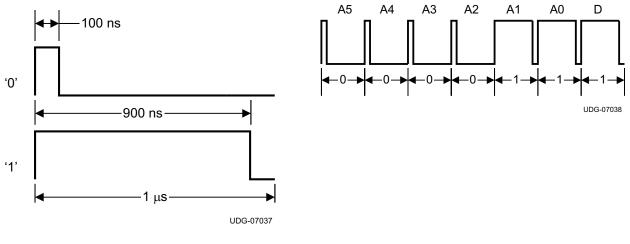
Figure 29. eTrim<sup>™</sup> Bit Pulse Timing
