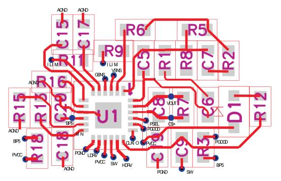
Figure 35. TPS40180 Recommended Layout for Peripheral Components
