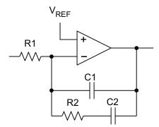
Figure 36. Type II Compensator
