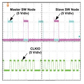
Figure 44. Switch Node and CLKIO Waveforms
