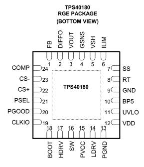
Figure 1. Device Pin Out
