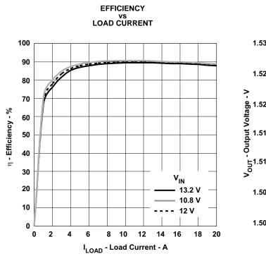
Figure 38. Efficiency Curve
