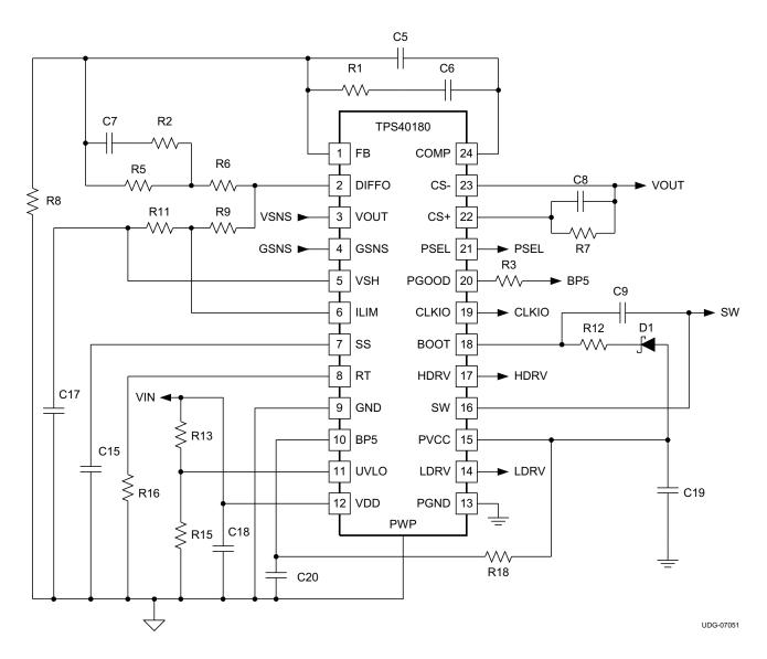
Figure 34. TPS40180 Peripheral Schematic
