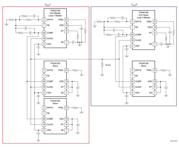
Figure 33. Multiple Multiphase Configuration
