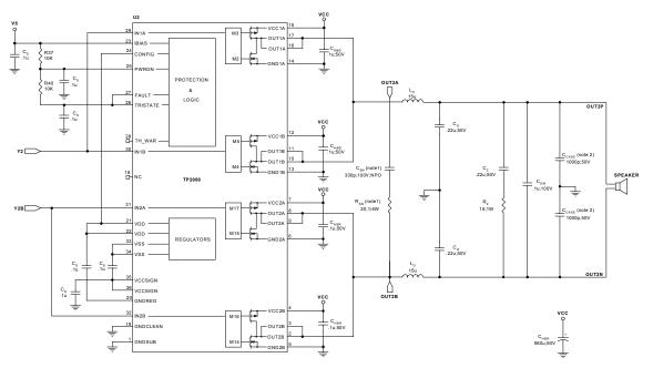
NOTE 1: C<sub>SN</sub>/R<sub>SN</sub> are optional locations, loaded only if required to reduce overshoot
