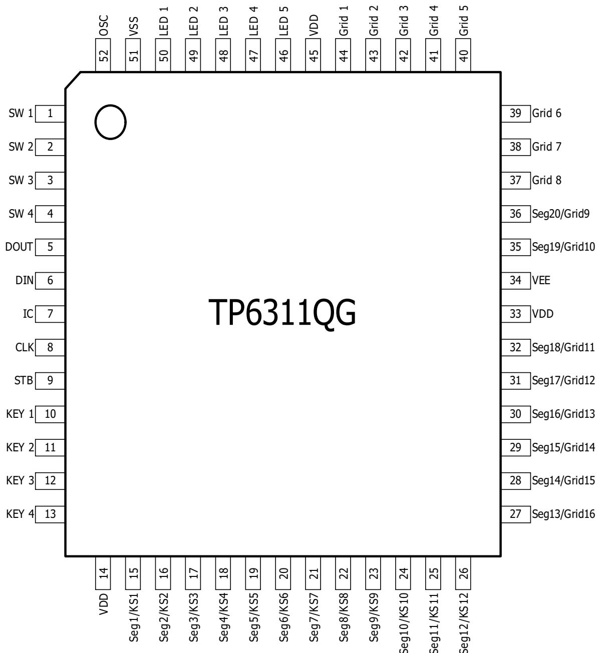
Use all the power pins. Leave the IC pin open.
