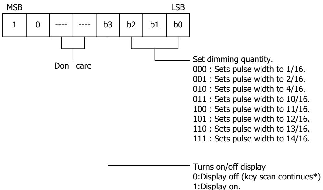
On power application, the 14/16-pulse width is set and the display is turned off.
