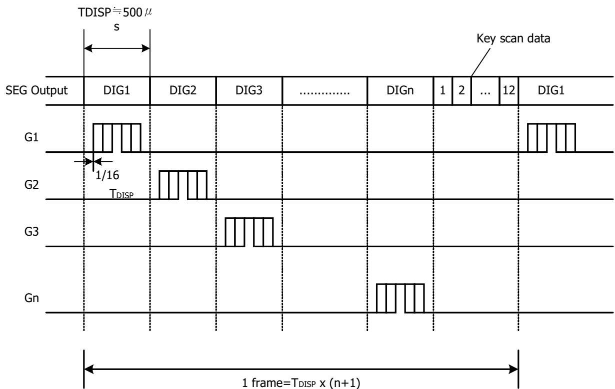
One cycle of key scanning consists of two frames, and data of  $12 \times 4$  matrices is stored in RAM.
