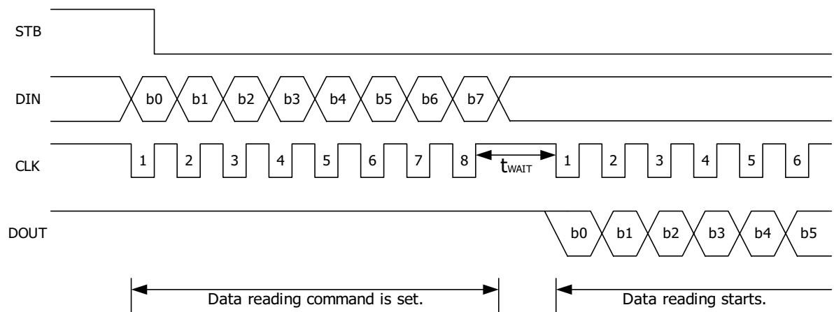
Because the DOUT pin is an N-ch, open-drain output pin, be sure to connect an external pull-up resistor to this pin (1k $\Omega$  to 10 k $\Omega$ ).
