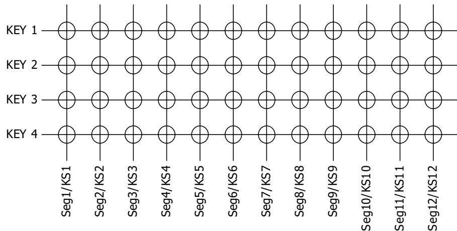
The data of each key is stored as illustrated below, and is read by a read command, starting from the least significant bit.
