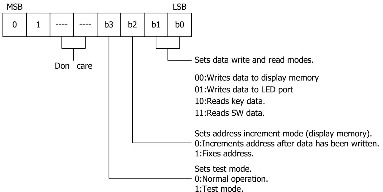
On power application, the normal operation mode and address increment mode set.
