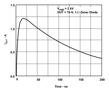
Figure 6. Typical HBM Current Waveform
