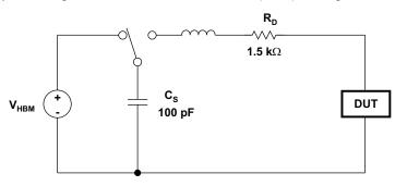
Figure 5. HBM ESD Test Circuit
