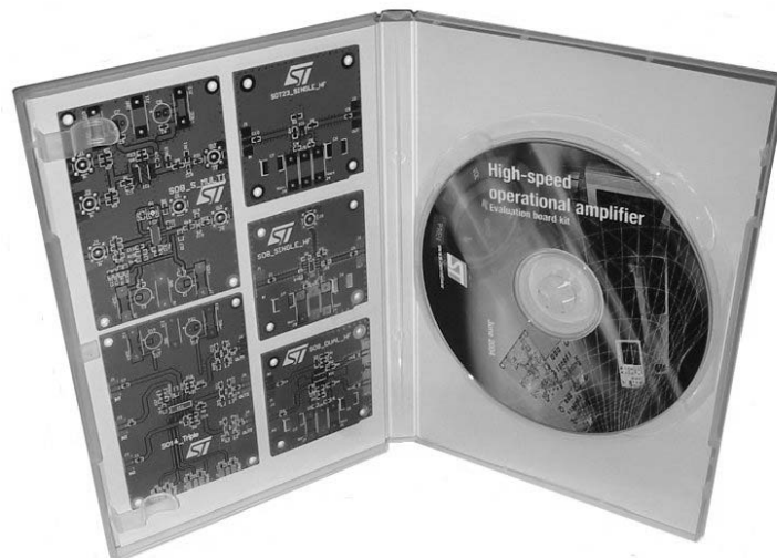
Figure 22: Evaluation kit for high speed op-amps
