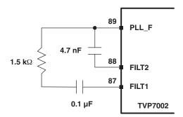
Figure 4. Horizontal PLL Loop Filter
