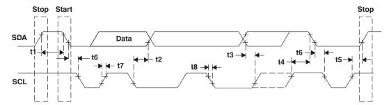
Figure 2. I<sup>2</sup>C Host Port Timing
