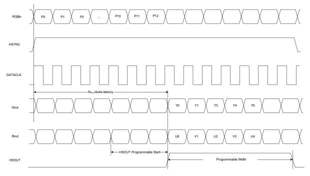
4:2:2 YCbCr Output Timing. Npd = 39 clock cycles. HSOUT start is programmable in register 21h.
