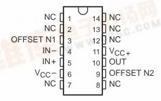
μΑ741M . . . JG PACKAGE μΑ741C, μΑ741I . . . D, P, OR PW PACKAGE (TOP VIEW)
