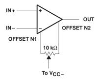
Figure 2. Input Offset Voltage Null Circuit
