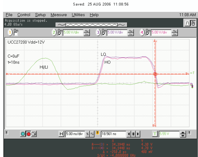
Figure 34. 10-ns Input Pulse Delay Matching
