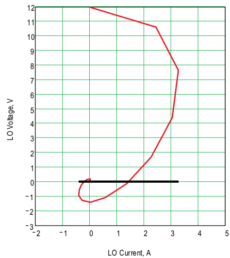
Figure 25. Turn-Off Voltage and Current Switching Diagram
