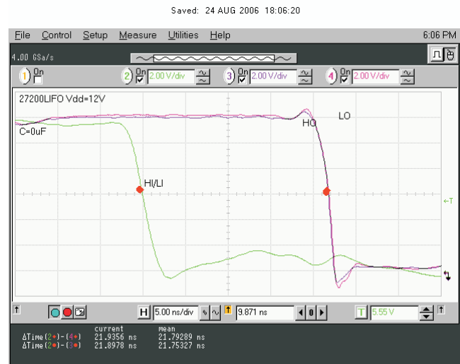
Figure 32. V_{LO} and V_{HO} Falling Edge Delay Matching
