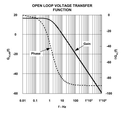
Figure 31. Bode Plot of the Open Loop Voltage Transfer Function
