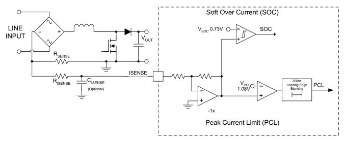
Figure 25. Soft Over Current (SOC) / Peak Current Limit (PCL)
