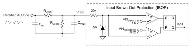
Figure 23. Input Brown-Out Protection (IBOP)
