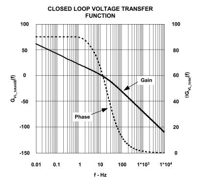
Figure 32. Closed Loop Voltage Bode Plot
