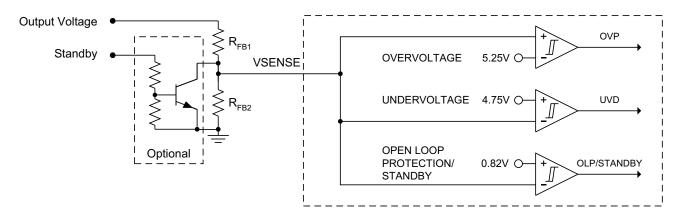
Figure 24. Over Voltage Protection, Open Loop Protection/Standby
