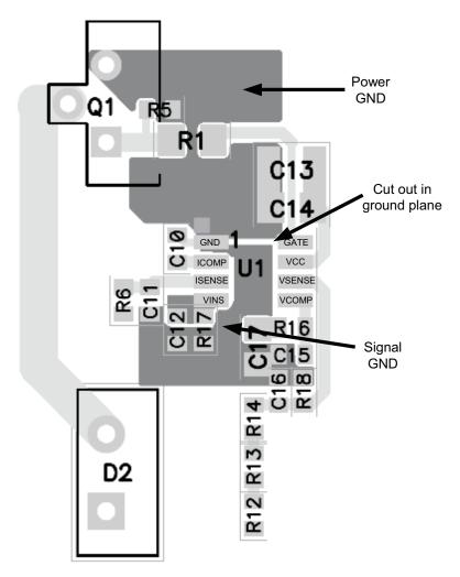
Figure 27. Recommended Layout for the UCC28019
