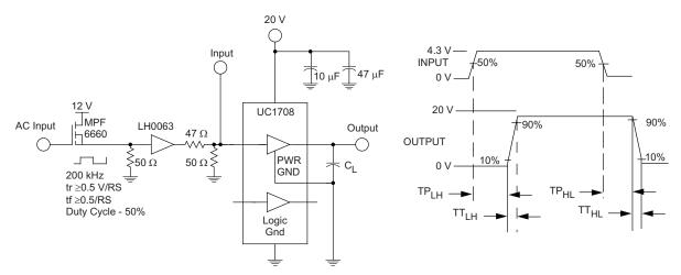
Figure 1. AC Test Circuit and Switching Time Waveforms
