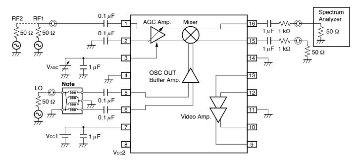
Note: Balun Transformer: TOKO 617DB-1010 B4F (Double balanced type)
