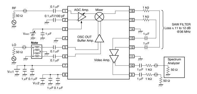
Note: Balun Transformer: TOKO 617DB-1010 B4F (Double balanced type)
