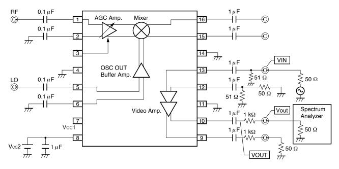
Voltage Gain(Single Ended) = 20Log(VOUT/VIN) (dB) Differential Gain(Differential-out) = 20Log(2\*VOUT/VIN) (dB)
