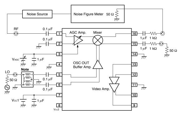
Note: Balun Transformer: TOKO 617DB-1010 B4F (Double balanced type)
