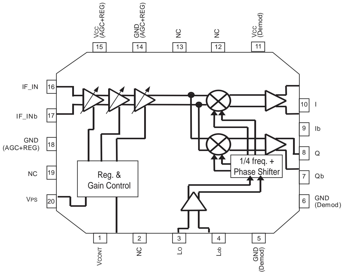
**PIN FUNCTIONS** (Pin Voltage is measured at Vcc = 3.0 V)
