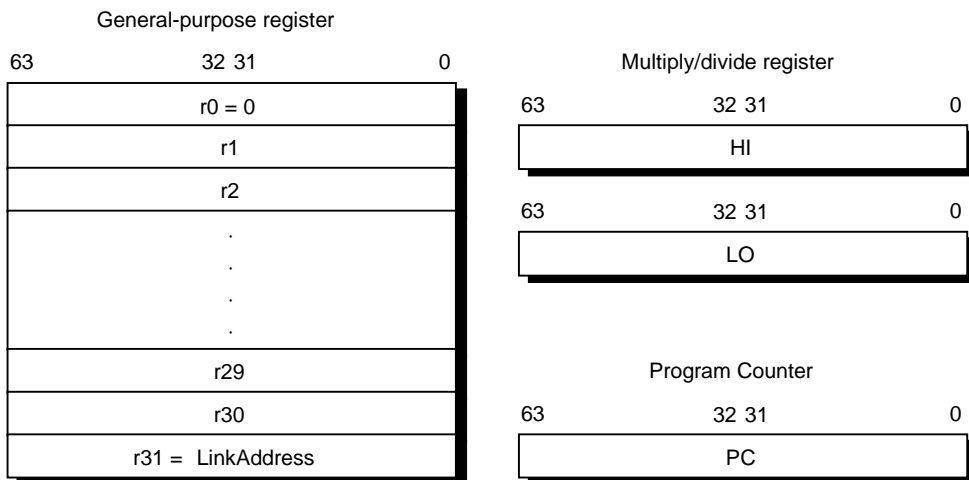
Figure 1-3. V R 4102 CPU Registers
