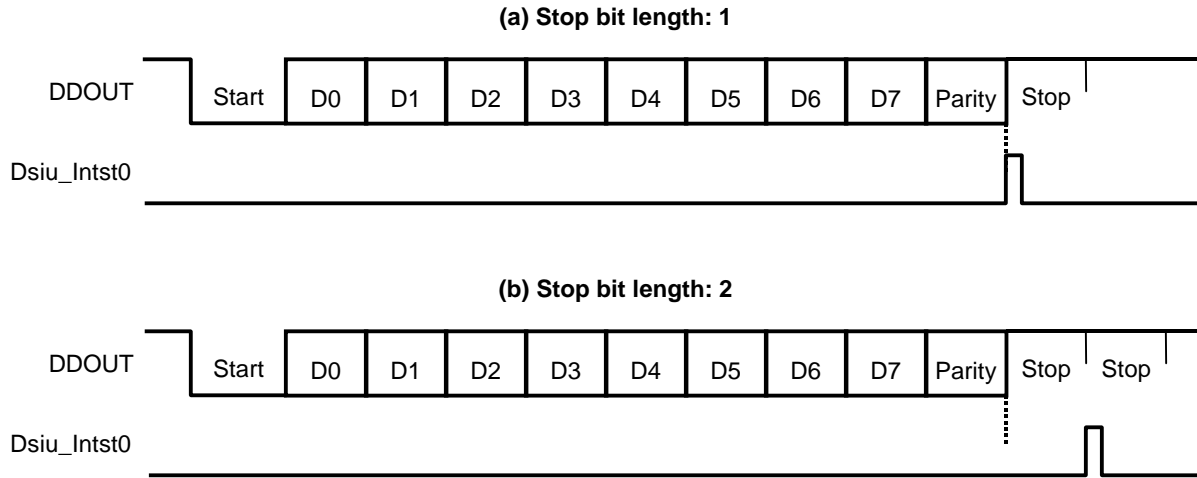
Figure 22-2. Transmit Complete Interrupt Timing
