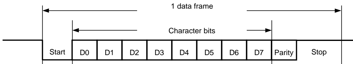
Figure 22-1. Data Format for Transmission and Reception
