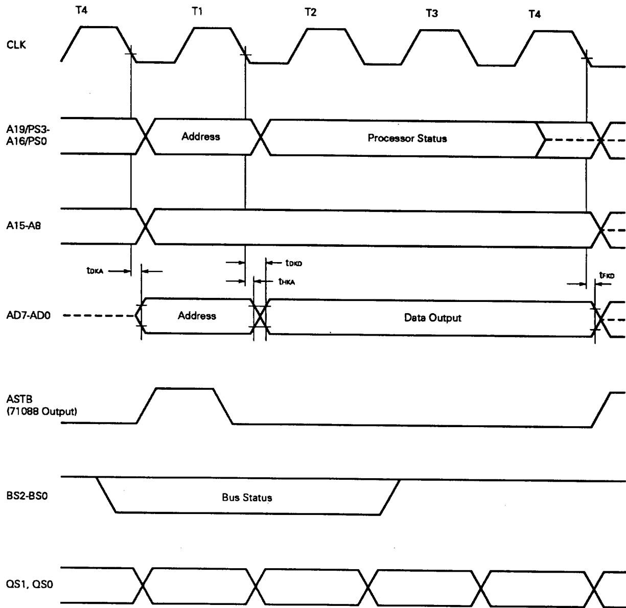
**Remark** A broken line shows high impedance.
