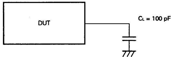
**Caution** If load capacitance exceeds 100 pF due to the configuration of circuits, lower the load capacitance to 100 pF or less by inserting a buffer, etc.
