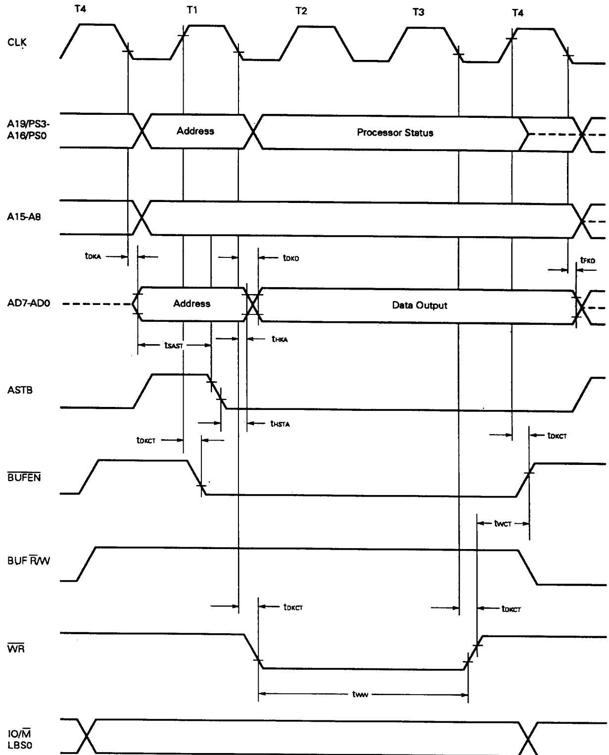
Remark A broken line shows high impedance.
