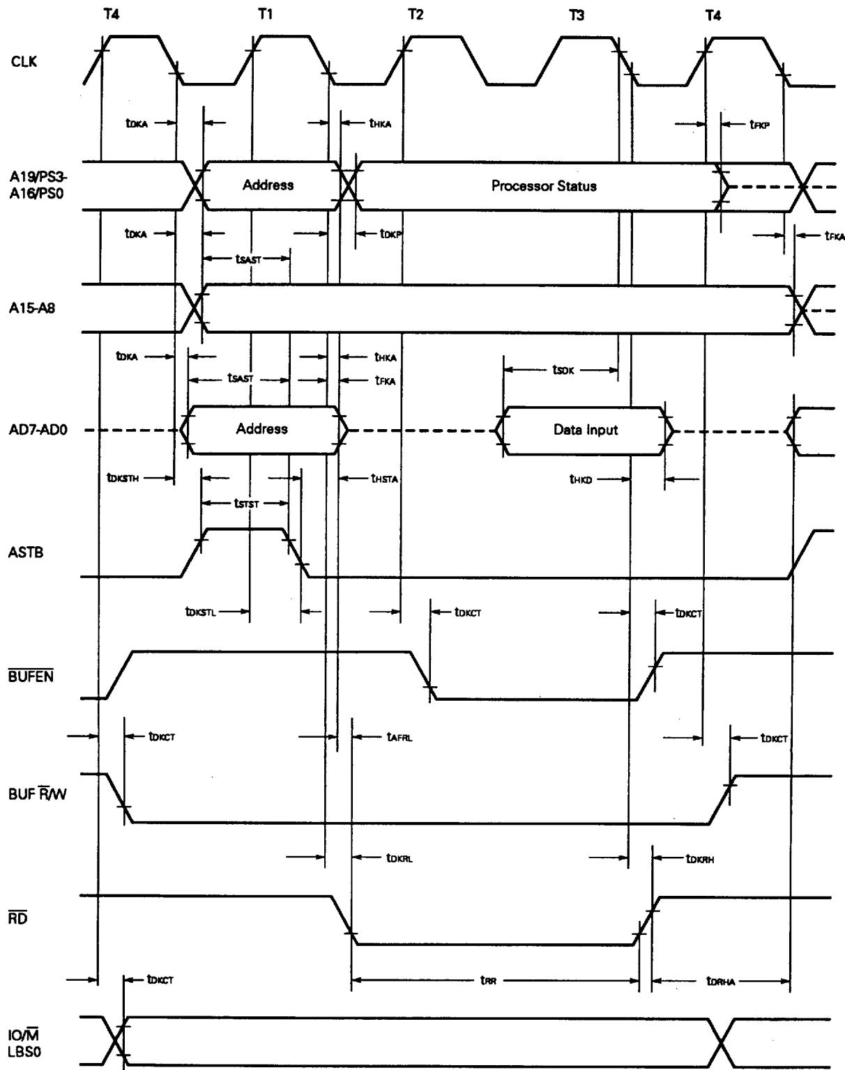
Remark A broken line shows high impedance.
