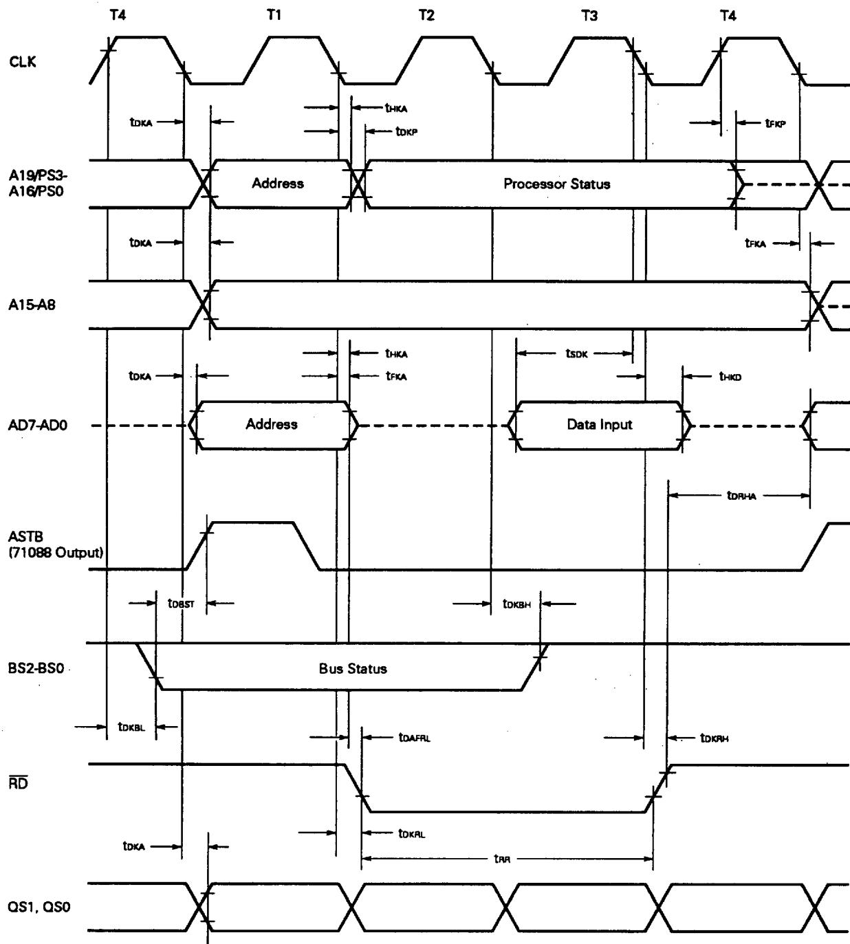
**Remark** A broken line shows high impedance.
