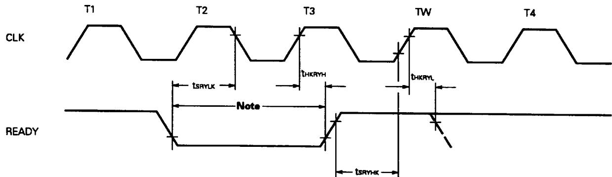
**Note** It is necessary to fix the READY signal to low (or to high) during this period.
