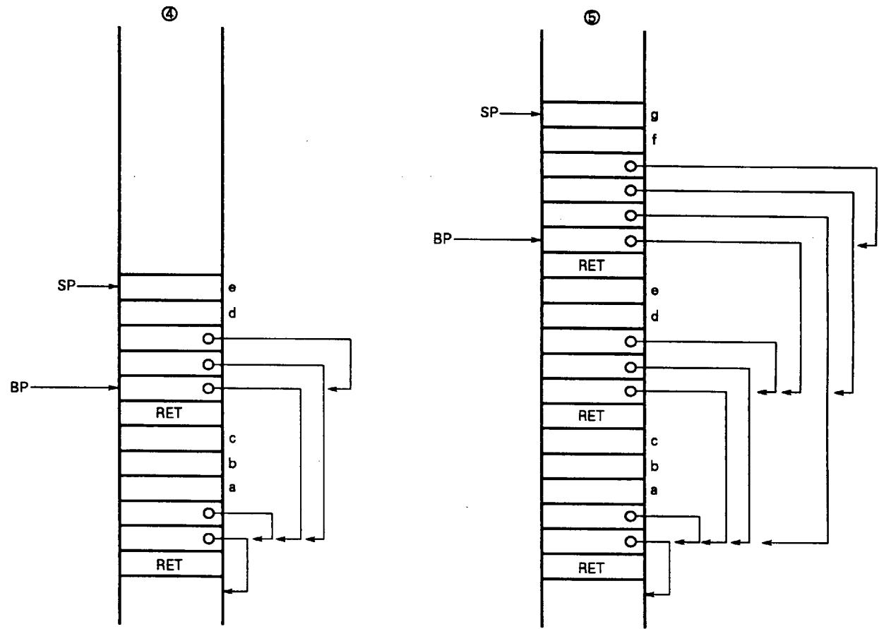
The PREPARE instruction saves BP to a stack first in order to restore the BP of a procedure at the called side when the procedure finishes. Then, it pushes a frame pointer (a saved BP) onto the stack within the range accessible from the called procedure. The accessible range equals to the value which is subtracted by one from the lexical level of the procedure.
