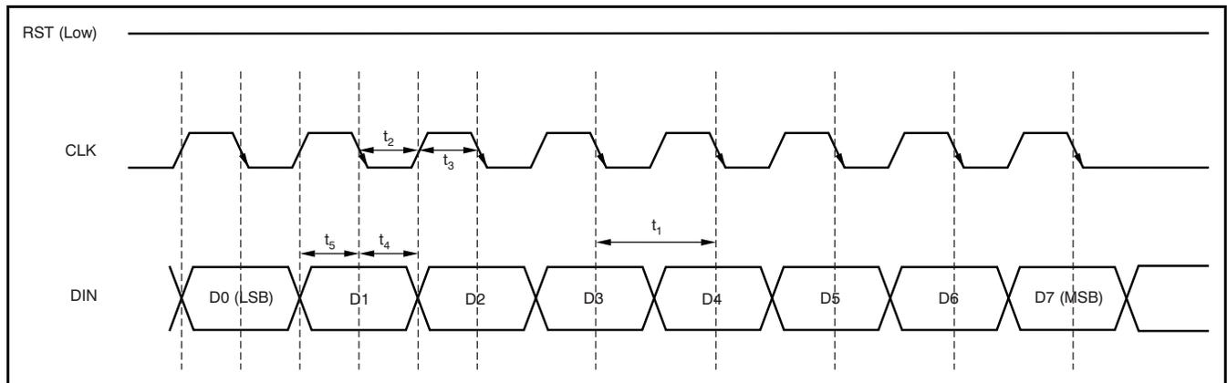
NOTE: This figure shows timing example for one data byte. A full register update cycle requires all five bytes (that is, 40 bits).
