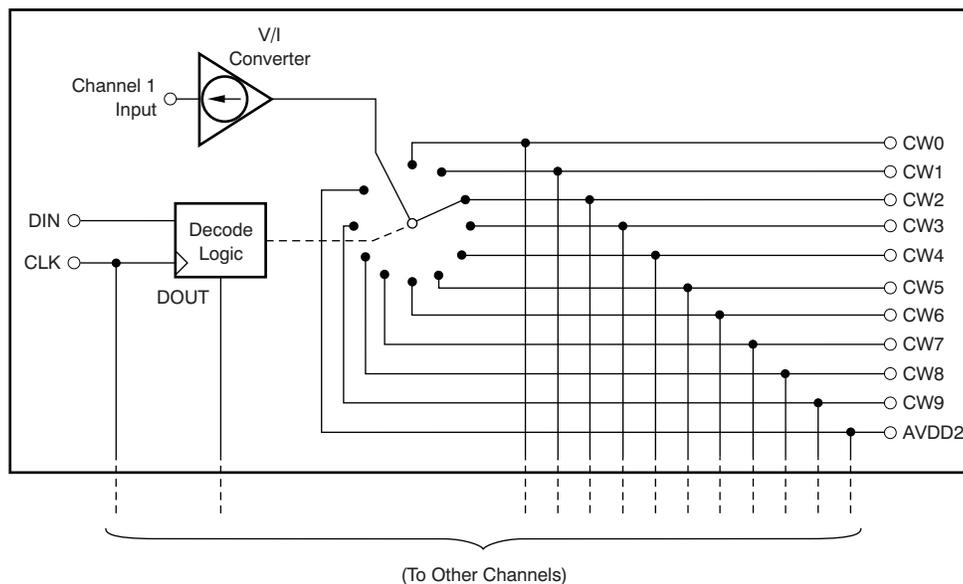
Figure 1. Basic CW Cross-Point Switch Matrix Configuration
