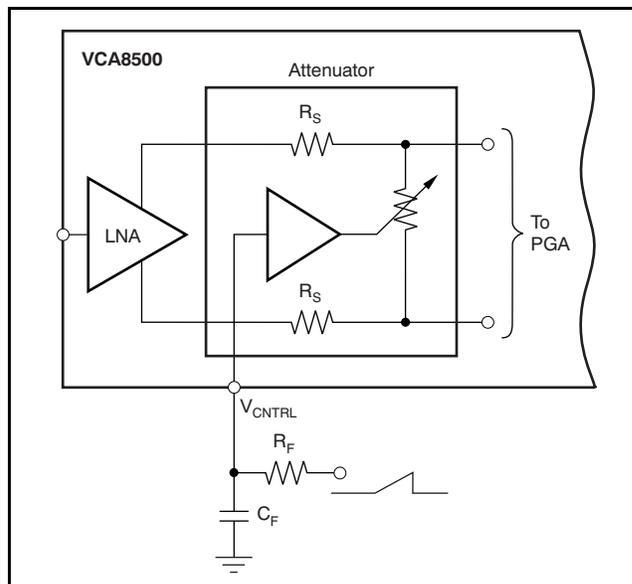
**Figure 66. External Filtering of the  $V_{\text{CNTRL}}$  Input**
