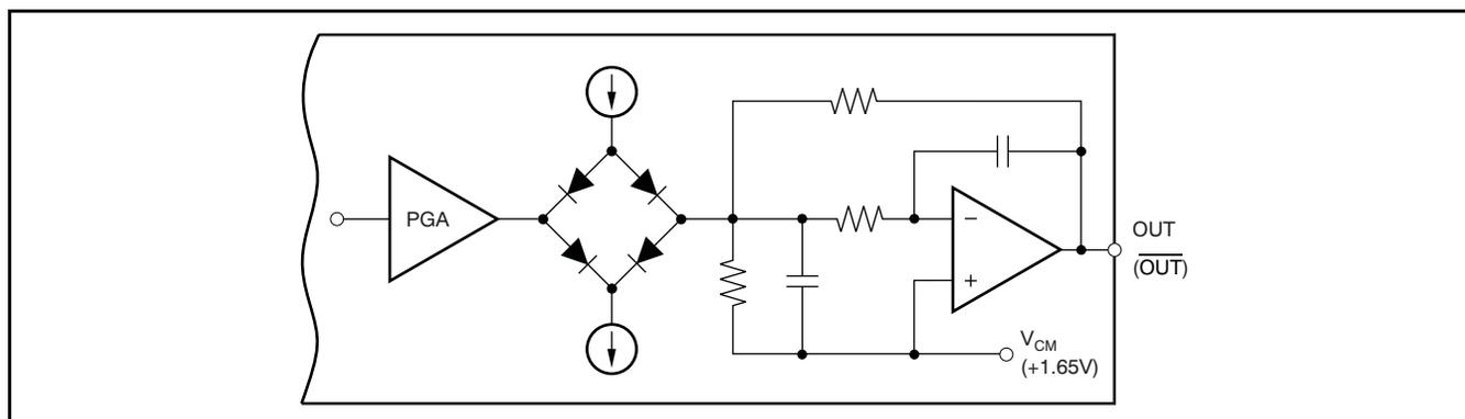
Figure 63. Clamping Stage and Low-Pass Filter (Simplified Schematic)
