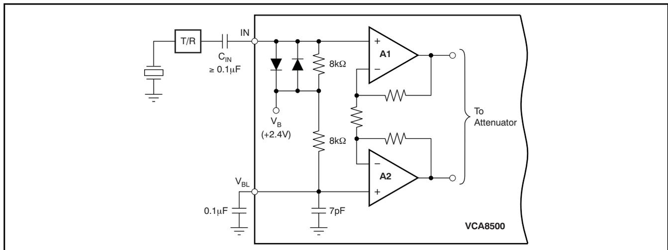
**Figure 64. LNA Channel (Simplified Schematic)**
