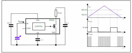
Figure 6. OVP threshold test circuits
