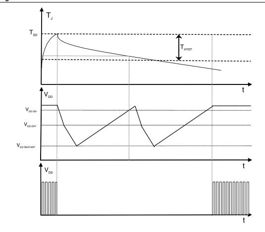
Figure 19. Thermal shutdown
