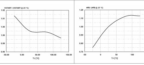
Figure 11. Brown out threshold vs T<sub>J</sub>
