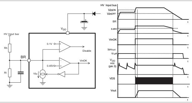
Fixed the  $V_{INon}$  and the  $V_{INoff}$  levels, with reference to *Figure 31*, the following relationships can be established for the calculation of the resistors  $R_H$  and  $R_L$ :
