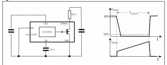
Figure 4. Minimum turn-on time test circuit
