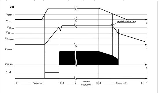
Figure 23. Timing diagram: normal power-up and power-down sequences
