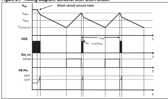
Figure 21. Timing diagram: behavior after short circuit
