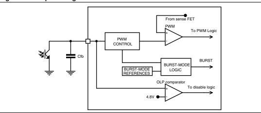
Figure 25. FB pin configuration
