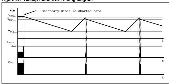
Figure 27. Hiccup-mode OCP: timing diagram
