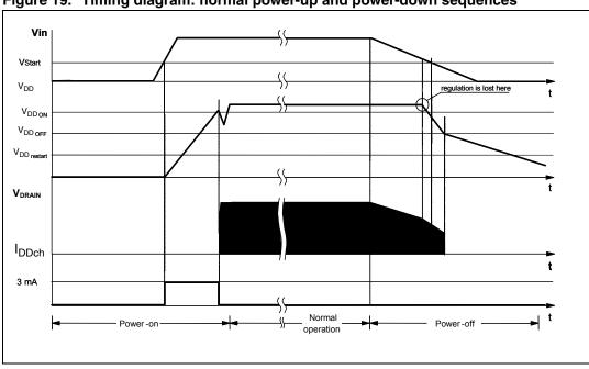
Figure 19. Timing diagram: normal power-up and power-down sequences
