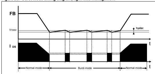
Figure 26. Burst mode timing diagram, light load management
