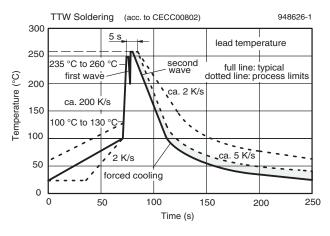
Figure 11. Double Wave Soldering of Opto Devices (all Packages)
