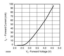
Figure 4. Forward Current vs. Forward Voltage
