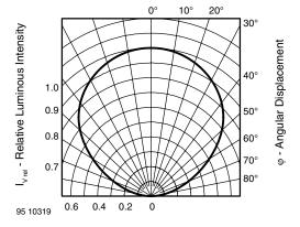
Figure 2. Relative Luminous Intensity vs. Angular Displacement
