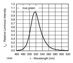
Figure 3. Relative Intensity vs. Wavelength
