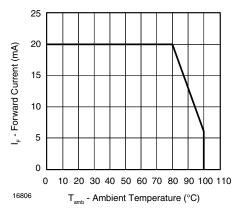
Figure 1. Max. Permissible Forward Current vs.
