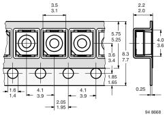
Figure 7. Tape Dimensions in mm for PLCC-2
