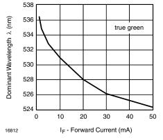
Figure 6. Dominant Wavelength vs. Forward Current
