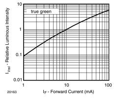
Figure 5. Specific Luminous Intensity vs. Forward Current
