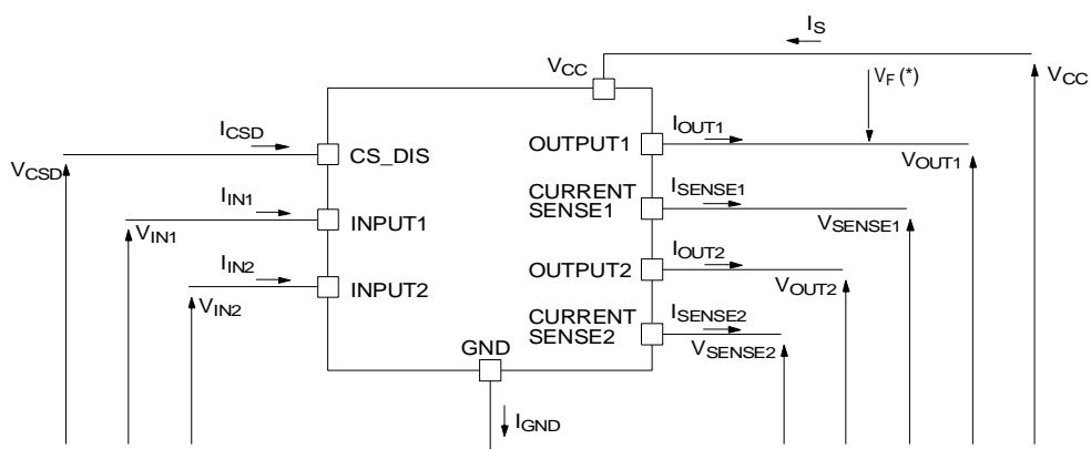
(\* )  $V_{Fn} = V_{CC} - V_{OUTn}$  during reverse battery condition
