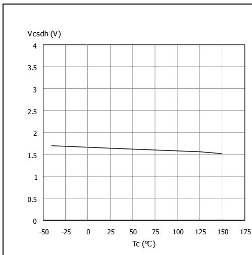
**Figure 23. CS\_DIS clamp voltage**
