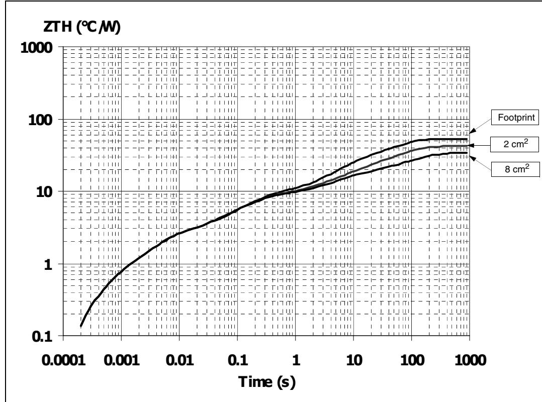
Figure 31. Thermal fitting model of a double channel HSD in PowerSSO-24<sup>(a)</sup>
