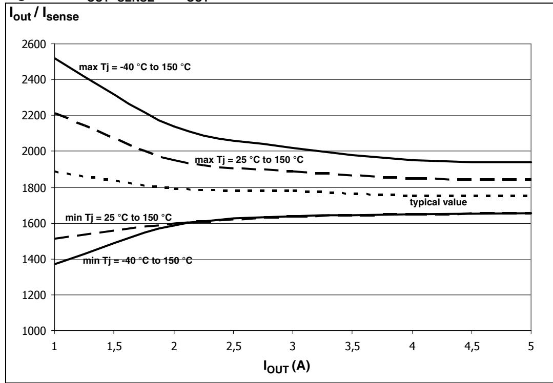
**Figure 8.** Maximum current sense ratio drift vs load current
