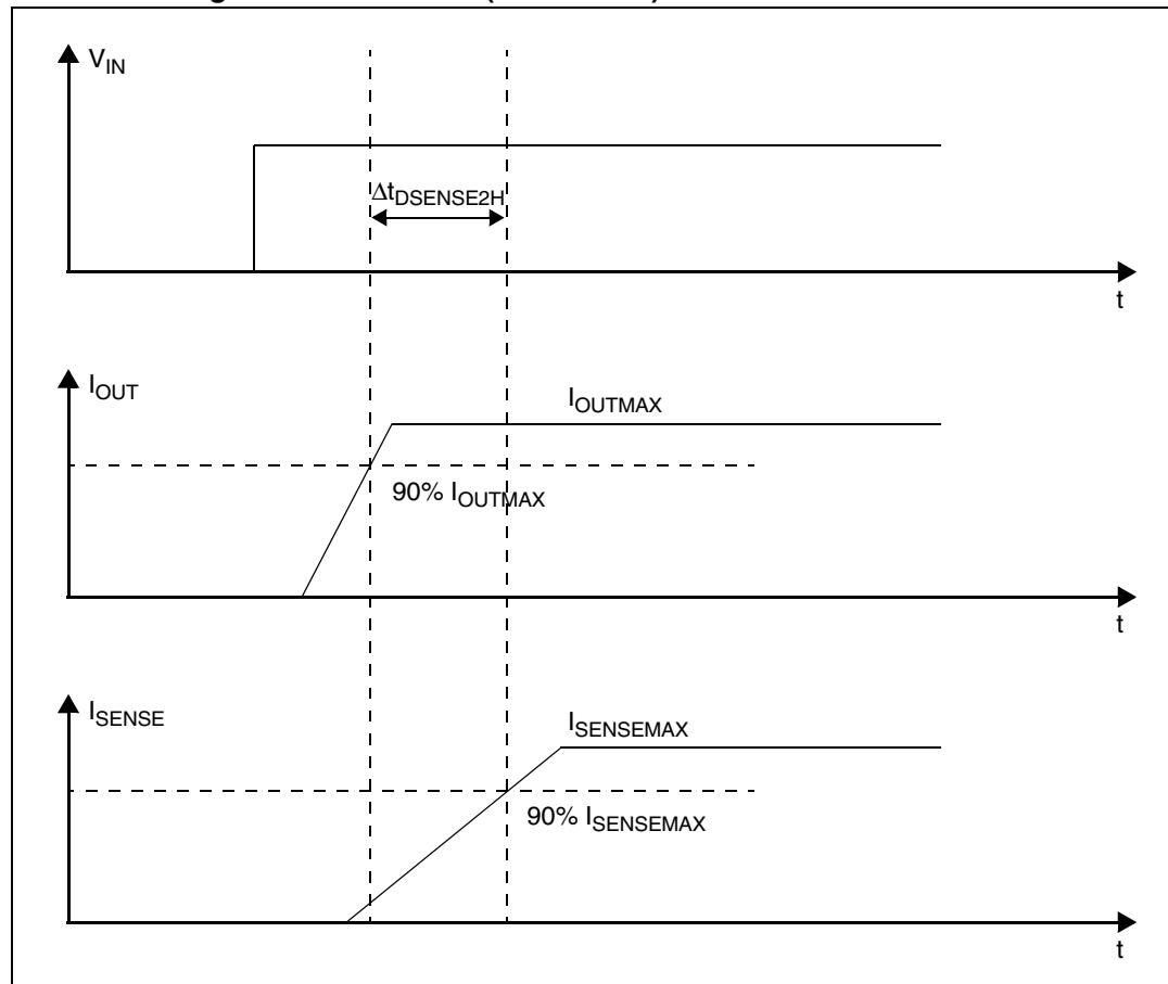
**Figure 6. Switching characteristics**
