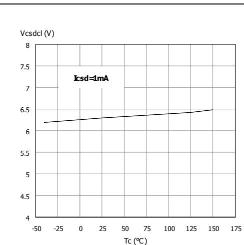
**Figure 24. CS\_DIS low level voltage**
