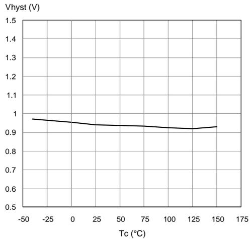
Figure 15. Overvoltage Shutdown
