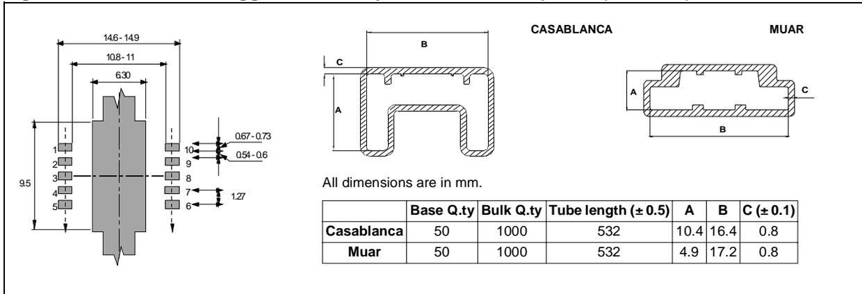
Figure 31. Tape And Reel Shipment (suffix “13TR”)
