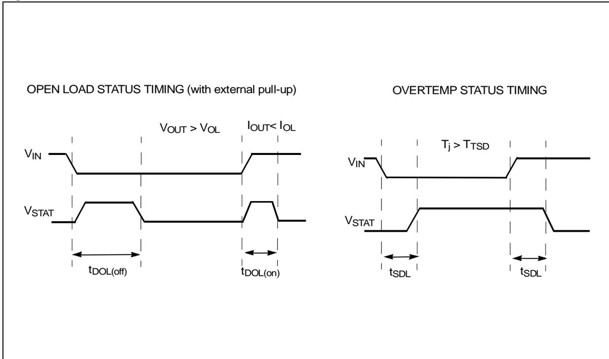
Figure 6. Switching time Waveforms
