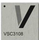
The VSC3104/3108 are multipurpose switching devices that are designed to enable next generation backplane designs, and extend the life of existing backplanes. The integrated equalization capabilities at both the input and output effectively absorb the effects of signal loss through copper interconnect, either printed circuit board traces, or cable.
