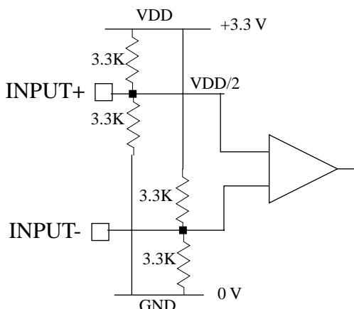
Because the VSC7121 output buffers are PECL outputs referenced to  $V_{DD}$ , the High Speed Differential outputs may not be direct coupled to the high speed differential inputs. One example of how to differentially cascade the two VSC7121 is shown in Figure 4. This circuit only applies if trace lengths are less than three inches.
