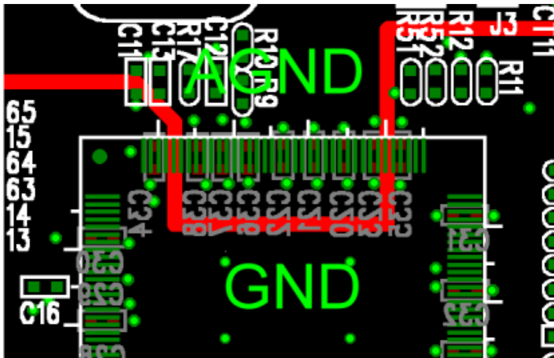
Figure 8. Reference Ground Partitions under the VT6202
