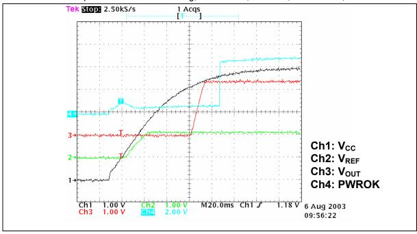
Power shut down with condition: no loading; CSS=0.1uF; VCC=5V; VOUT=2.5V; f = 200 KHz.
