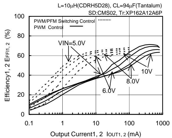
**FOSC=500kHz, VOUT1, 2=3.3V**
