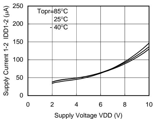
(7) Supply Current 2 vs. Supply Voltage
