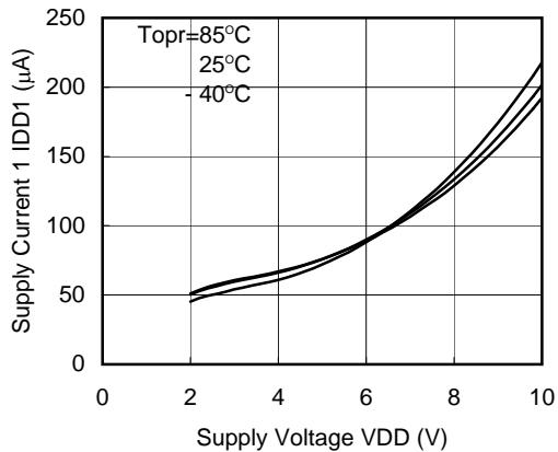
(5) Supply Current 1\_1 vs. Supply Voltage
