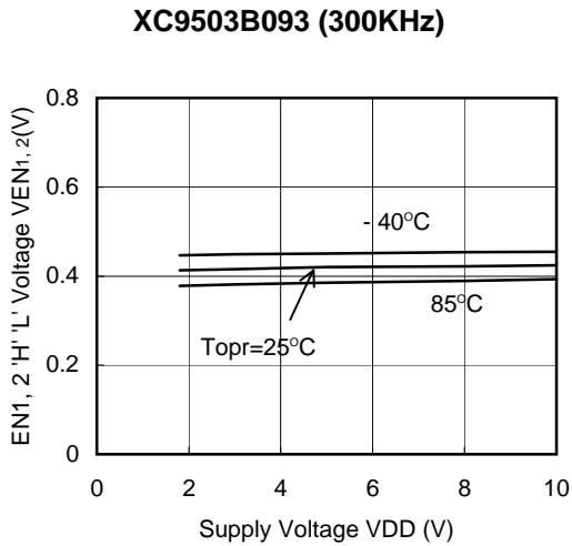
(11) PWM1, 2 'High' 'Low' Voltage vs. Supply Voltage
