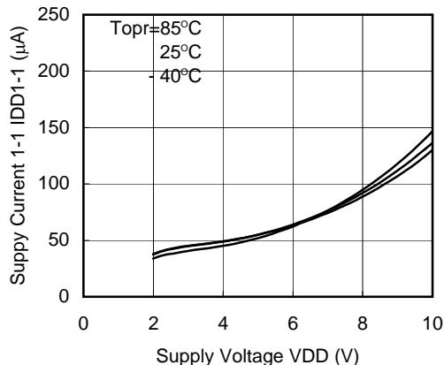
(6) Supply Current 1\_2 vs. Supply Voltage
