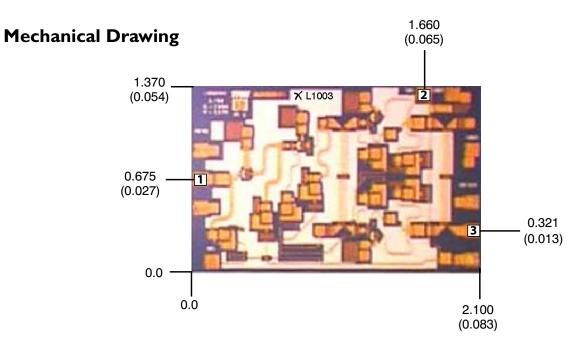
Units: millimeters (inches) Bond pad dimensions are shown to center of bond pad. Thickness: 0.110 +/- 0.010 (0.0043 +/- 0.0004), Backside is ground, Bond Pad/Backside Metallization: Gold All Bond Pads are  $0.100 \times 0.100 (0.004 \times 0.004)$ .
