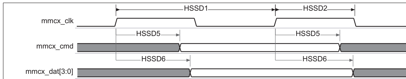
Figure 6-65. MMC/SD/SDIO – High-Speed SD Mode – Data/Command Receive
