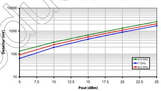
XP1035-QH: Detector (mV) vs Pout (dBm) at Id=500mA, Vd=6V, +80 C
