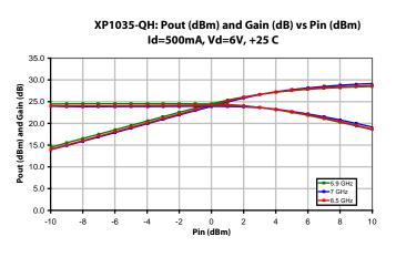
XP1035-QH: P1dB (dBm) at Id=500mA, Vd=6V
