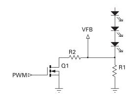
MOSFET 'off'  $I_{LED(MIN)} = \frac{V_{FB}}{R_{LED}}$
