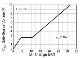
Gate-Source Voltage v Gate Charge
