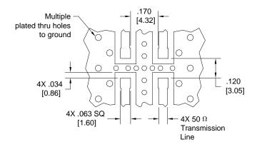
Dimensions are in Inches [Millimeters] 1P620\* Rev A Mounting Footprint
