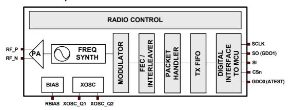
Figure 2: **CC2550** Simplified Block Diagram
