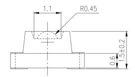
For reflow soldering (propose)
