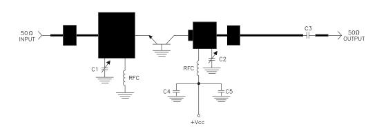
= Microstrip on 0.010" Duroid, Er=2.3 C1 = 0.6-6.5pF JOHANSON VARIABLE C2 = 0.3-3.5pF JOHANSON VARIABLE C3 = 82pF ATC CHIP CAP C4 = 82pF ATC CHIP CAP C5 = 2000 mFD
