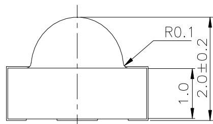
For reflow soldering (propose)
