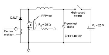
Fig. 8 - Unclamped Inductive Test Circuit
